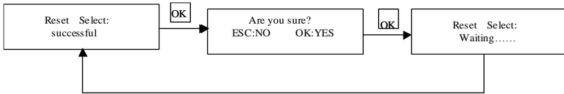
When the network control card is swapped or changed, the device will need to be reset. It is recommended to restore the default settings when changing the network control card.
