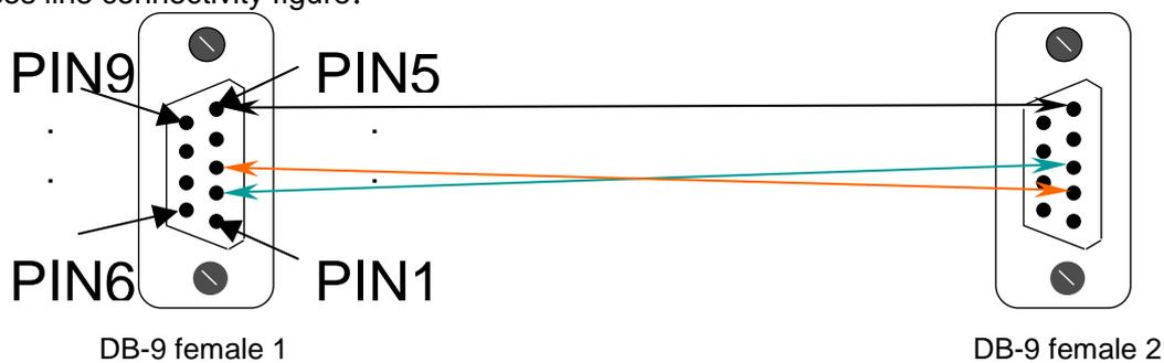
Figure 3-2 DB-9 cross connection layout
