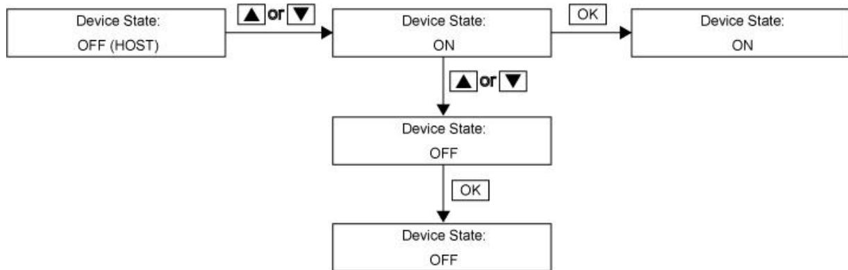
“Device State” setting is to open or close the function of redundancy. The default setting of “Device State” is OFF.
