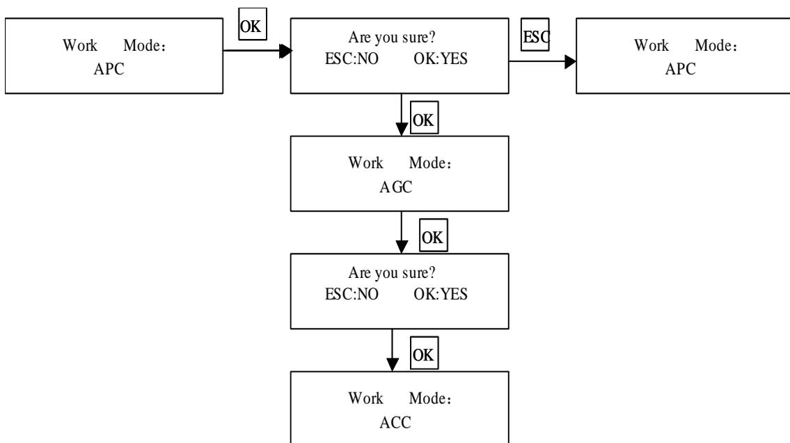
**Notice:** The equipment is already calibrated. There are no calibration settings for the optical output in different work modes. The output power may be incorrect when if the work mode is changed. Consult a PBN representative before making changes to the work mode.
